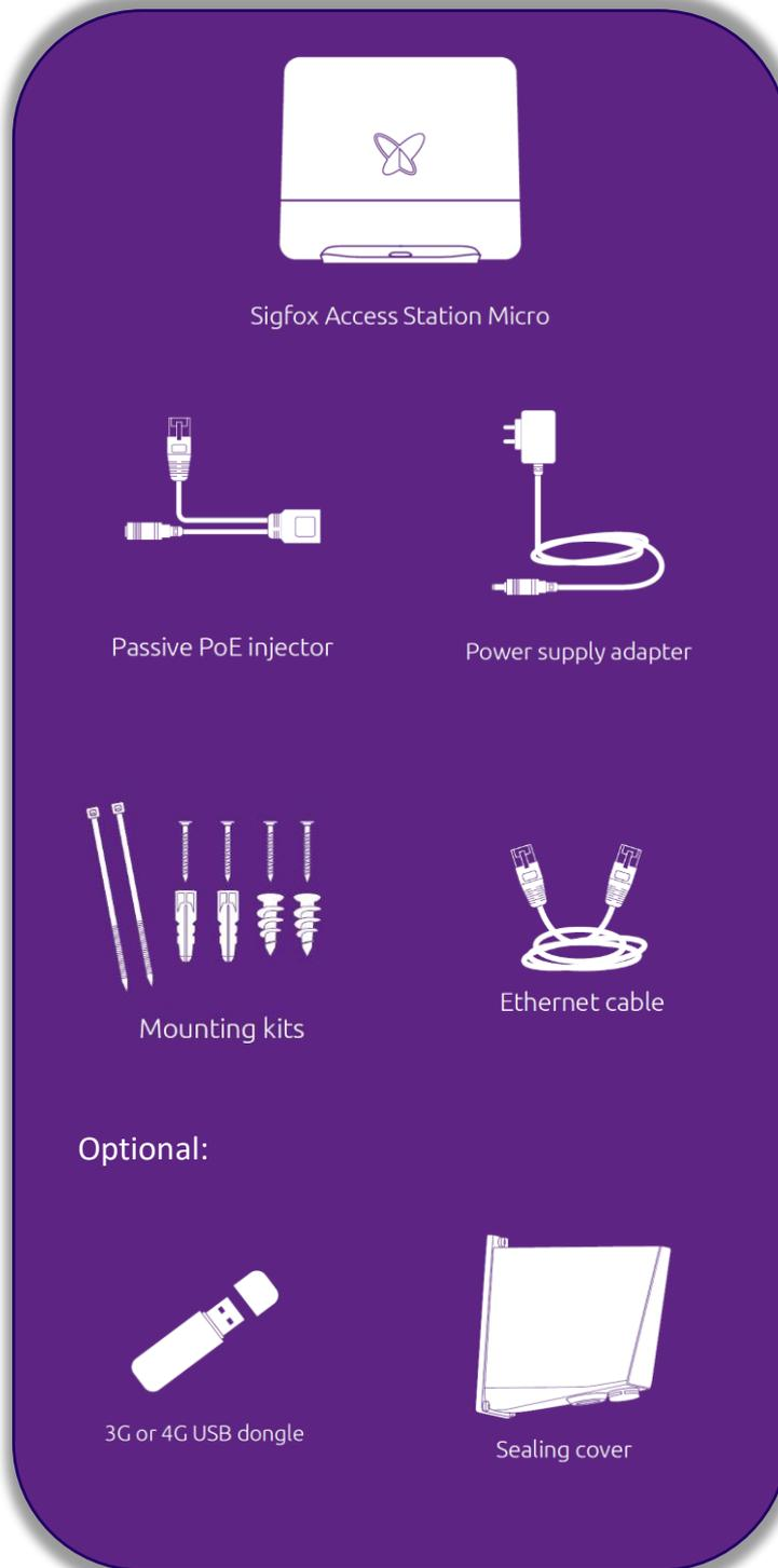
The diagram shows the contents of the Micro Station(s) package, arranged in a purple rounded rectangle. At the top center is the Sigfox Access Station Micro. Below it are two rows of accessories: a Passive PoE injector and a Power supply adapter. The next row contains Mounting kits and an Ethernet cable. The bottom section is labeled 'Optional:' and contains a 3G or 4G USB dongle and a Sealing cover.
